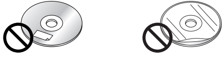
Disc with adhered stickers or tape Labels created by a printer or tape
